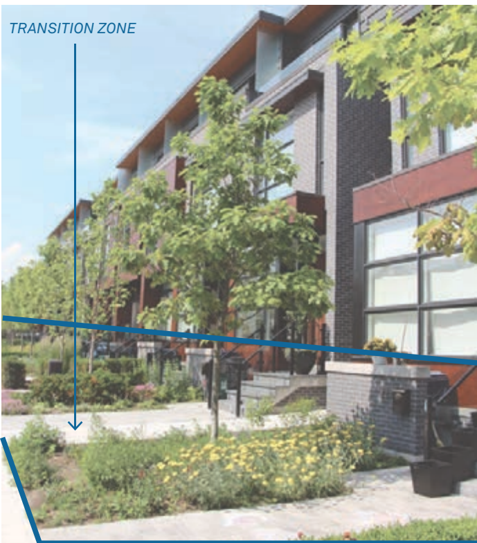
Landscape, a low wall and a grade change establish a transition to private space from the public sidewalk. (Image Credit: Brook McIlroy)
